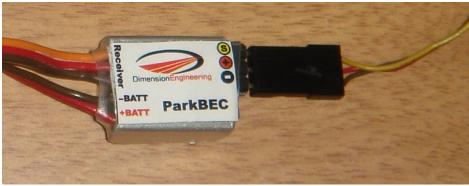
**Step 3:** Plug the radio connector of the **ParkBEC** into the throttle port of your receiver.
